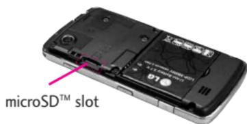
1. Remove the back cover and locate the microSD™ slot on the left side.
